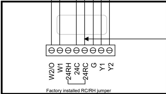
Most Heat Pump systems have the C wire and the thermostat can be powered by the 24VAC from the HVAC system.
