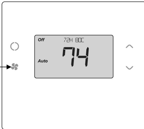
Press and hold the FAN button for 5 seconds to go to the Menu Mode screen
